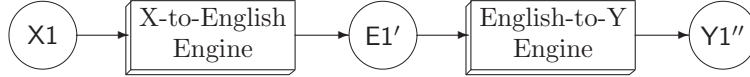
Figure 4: The concept of error accumulation. The X-to-English translation engine may produce English sentences with some errors. Regardless of the existence of errors in the intermediate English, also the English-to-Y engine causes some errors, thus the quality of Language Y is worse than that of English.
